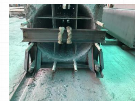
柱顶、柱底工装
