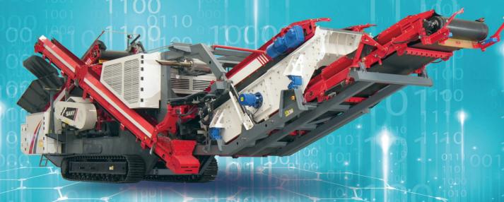
It is used for secondary and tertiary crushing and recycling of hard materials with compressive strength not exceeding 300Mpa in construction transportation, railway, cement, building materials, metallurgy, tailings and other industries.
